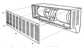
Figure 3 - Removing Air Intake Grille
